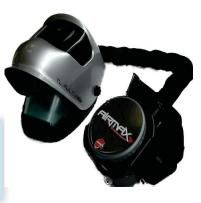
Self heating system kit "suitable for welding and grinding"; It is made of a filtering belt unit, complete with lithium battery (8/10 hours), battery charger, TH2PSL filter, belt, proban connecting hose to the mask. transparent protection visor with tip up front visor with adiactinic glass DIN 10 dim. 110x90mm.
