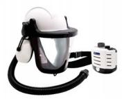
The kit consists of a case containing: helmet complete with headphones and adjustable anti-fog visor, battery and battery charger with 4 types of plugs, 7.4V light lithium ions, 200 liters of filtered air per minute, TH2PSL particulate filter and 5 prefilters lasting 8/10 hours.
