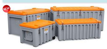
Box made of high-grade PE suitable for transport and storage of tools and small parts. Optimal dimensions for flatbed vehicles, stackable, with locating lugs and recesses and forklift pockets. Integrated handles, lid with upper beating toggle latches, space for label pocket. Water ingress prevented by integral seal around entire lid. Weight: 30 Kg.
