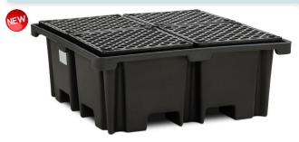
Collecting trays for PE drums with general building inspection approval Z-44.22-574 and Z-40.22-579. Made of polyethylene (HDPE), high chemical resistance. The trays can be placed directly on the floor, equipped with integrated fork holes. Accessible on all four sides. Loaded pallets can be arranged with stackers or forklifts directly on the trays. Complete with PE grid (various grills on request).
