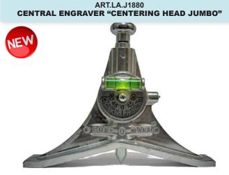
The central engraver is used for tubes starting from diameter of cm. 2.5 and over. In the engraver there is an adjustable stop rod and a protractor with bubble. After having extracted it to the stop point and after having leveled the engraver, release the rod by pressing the locking spring. The pressure exerted on the rod will strongly hit the tube marking the center.
