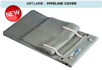
Special protection cover for controlled cooling of pipe welds. Prevents from thermal shock and protects the welding cord from external agents. Quick coupling and release system with belt and fixing buckle. Covered externally in water-repellent polyurethane, internal fabric resistant up to 600 ° C. Standard width 300mm, variable diameters from 200 up to 1400mm. Packing: 1/1.
