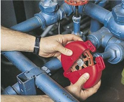
It encloses the entire valve, so it can no longer be opened or closed. The V-SAFE valve cover consists of two flattened half moons that completely cover the valve. Made of dielectric polypropylene, extremely resistant to scratches and abrasions, resistant to sudden changes in temperature. Dimensions: up to diam. 2.5".
