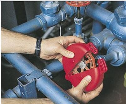
It encloses the entire valve, so it can no longer be opened or closed. The V-SAFE valve cover consists of two flattened half-moons that completely cover the valve. Made of dielectric polypropylene, extremely resistant to scratches and abrasions, resistant to sudden changes in temperature. Dimensions: from 5 "up to 6.5".
