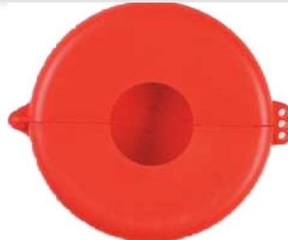
It encloses the entire valve, so it can no longer be opened or closed. The V-SAFE valve cover consists of two flattened half-moons that completely cover the valve. Made of dielectric polypropylene, extremely resistant to scratches and abrasions, resistant to sudden changes in temperature. Dimensions: from 2.5 "up to 5".
