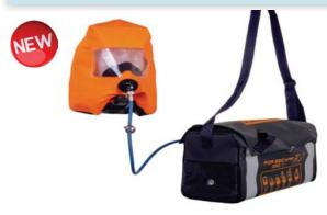
BIO-S-CAPE is an emergency compressed air device, intended for evacuation in toxic environments, fumes, insufficient oxygen fire. Hood with wide field of view, adaptable to all conformations. Manometer always visible. The positive pressure of the hood eliminates any risk of inhalation of toxic gases. Resistant to temperatures 0,1/+40,3 C. 2 LT air cylinder. 200 bar. (15 minute).
