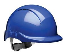
Helmet ABS (Acrylonitrile-Butadiene-Styrene). Short, ventilated peak, textile harness with 6 attachment points. Rear wheel ratchet regulator, antisweat band. Electrical insulation up to 1000V, Impact resistance up to - 40 °. Weight: g 329. (also available with integrated CE.S10 plus visor). Size: universal. Norms: CE EN 397:1995+A1 EN 397:2012+A1:2012 EN 50365 - ANSI/ISEA Z89.1-2009 Type 1
